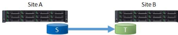
Figure 4-12 One-Directional Remote Replication
